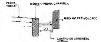
**DETALHE CANALETA SEM ESC.**
